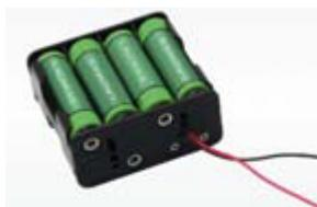
Battery pack made up of 8 NiMH rechargeable elements, 1.2 V, AA type
